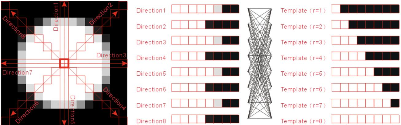
Figure 2. The circular-symbol detection algorithm
