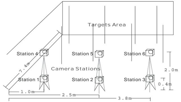
Figure 5. The distribution of exposure stations.
