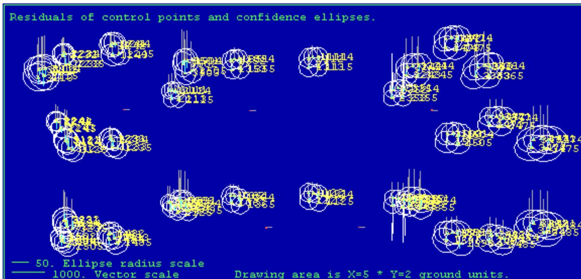
Figure 7. Residuals of points and confidence ellipses when object coordinates were treated as unknowns.
