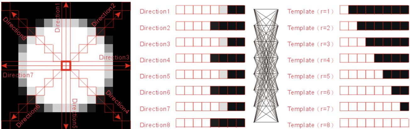
Figure 2. The circular-symbol detection algorithm
