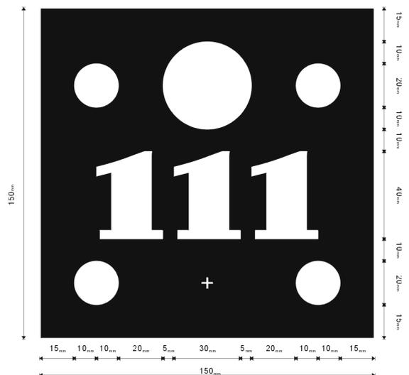
Figure 1. The proposed pattern of text-coded target
